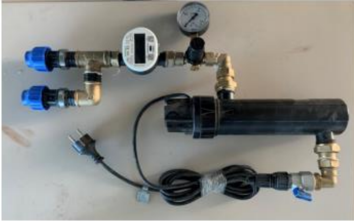
Figure 3-7c: VCA for water supply by pressure water: Photo (version with pressure water bypass to a next section downstream)
