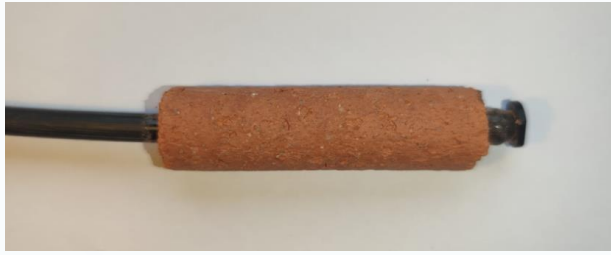
Figure 3-4a: SLECI-element with connectors to 6 mm hoses (branch-line) for Type A
