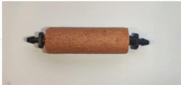
Figure 3-4b: SLECI-element with connectors to 6 mm hoses (double ended) for Type B
