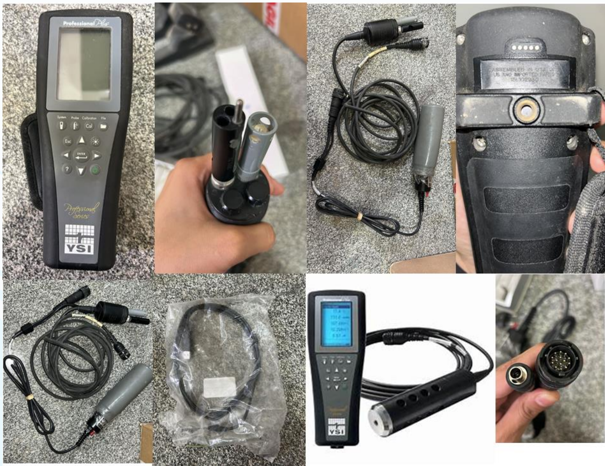
Figures 2. Demonstration of the Professional Plus water quality in-situ kit components and tools used for the water quality analysis
